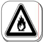
Gasoline is extremely flammable. Never expose the machine to a spark, open flame, high heat source, etc. that may present a fire hazard.
